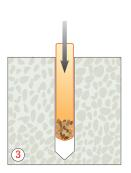
Insert Spin-In Capsule into drilled hole with air gap in capsule nearest to surface
