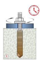
Allow the resin to cure for appropriate time. Attach fixture and tighten anchor to Recommended Torque
