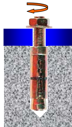
Position fixture, attach nut and washer and tighten to Recommended Torque
