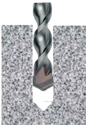
Drill correct diameter hole to correct depth
