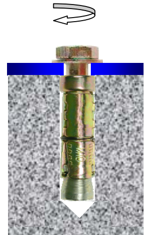
Position fixture, insert bolt and tighten to Recommended Torque
