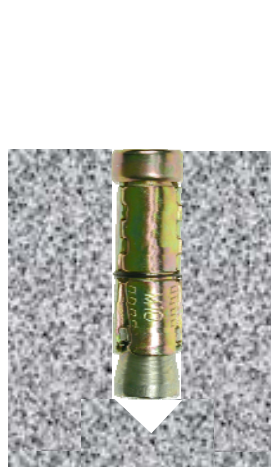
Insert shield into concrete
